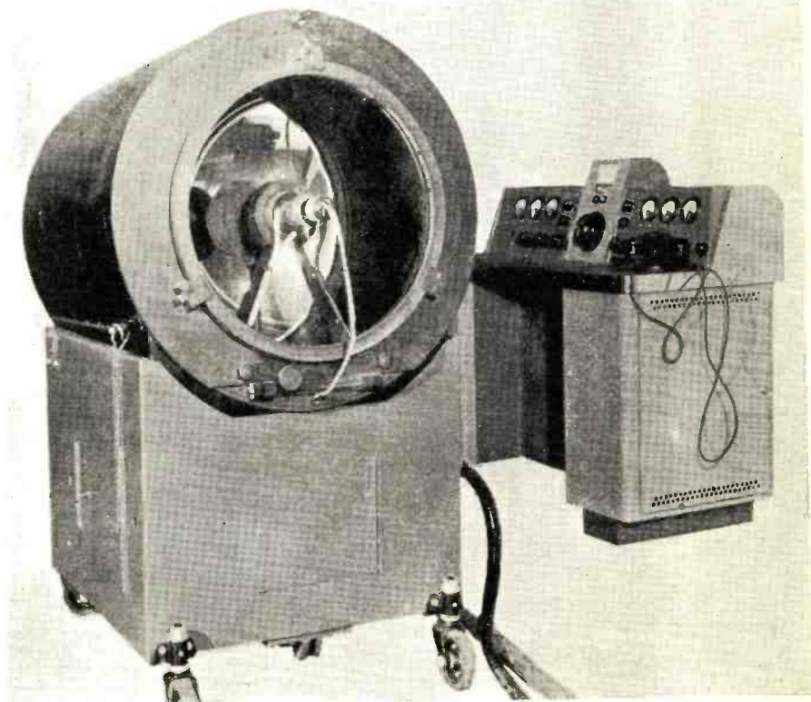
Fig. 3. Projector for theater television with control console in the background.
