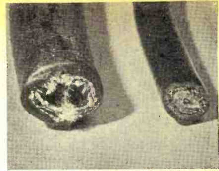
Fig. 4. Two types of coaxial cables occasionally used for TV antenna lead-ins in noisy urban locations.
