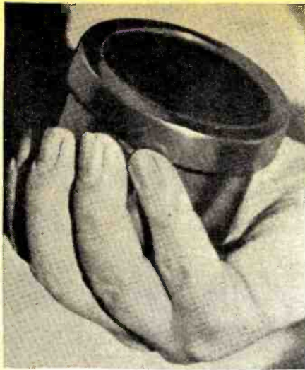
Fig. 4. Moving coil (dynamic) microphone.
