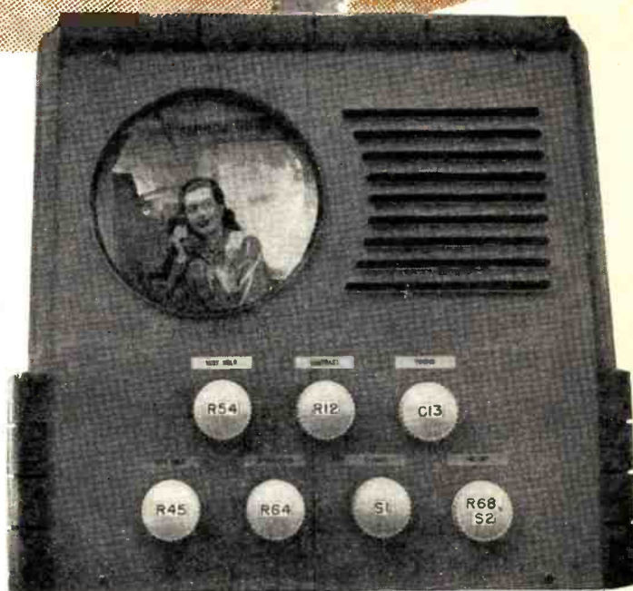
Front panel view of television receiver. The cabinet was home constructed. Controls from left to right are: (top) vertical hold, contrast, tuning, (bottom) horizontal hold, brightness, channel, and volume.
