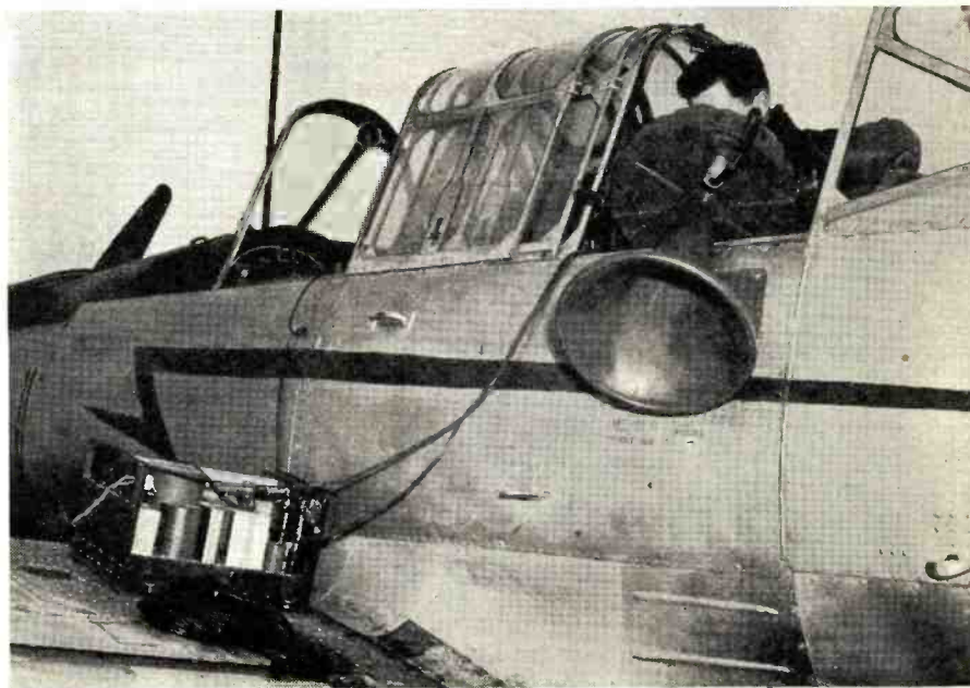
A Consolidated Vultee AT-6, purchased by an ex-AAF pilot from Army surplus, is shown being equipped with a University Model B-6, 150 watt loudspeaker unit.
