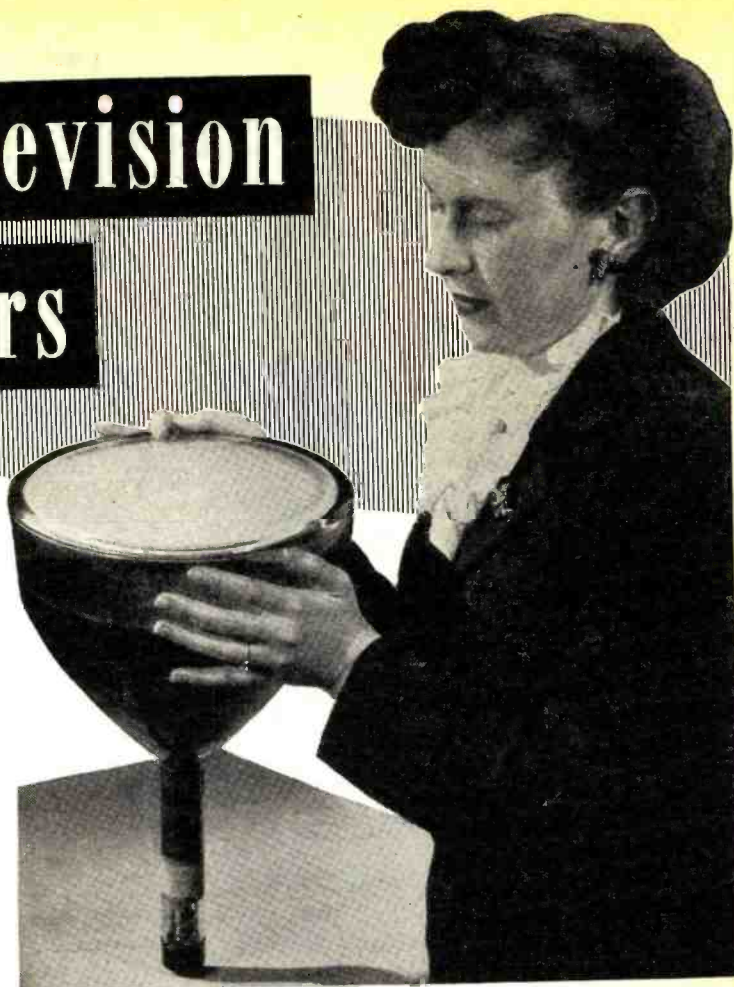
All video tubes are implosive by nature. The larger they are the more dangerous they become and therefore should always be handled with care.
